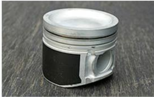
Fig 1.2 Dished Piston for Diesel Engine
