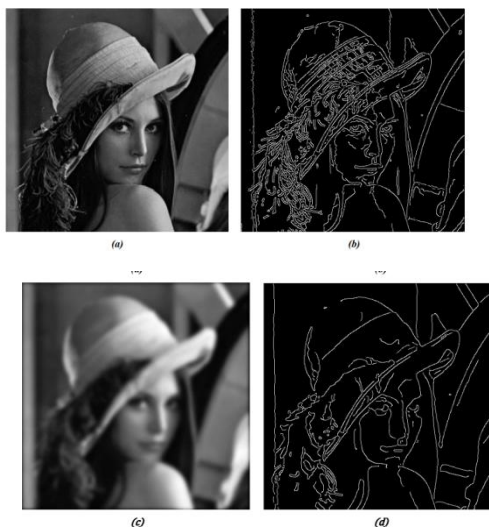
Figure 4.1 (a) The original Lena image; (b) Canny edge of the original image; (c) P-M diffused image after 60 iterations with static scale \lambda=65 ; (d) Canny edge of P-M diffused image.
