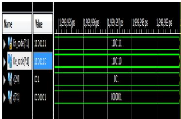
Fig.5 Hamming Code Decoder output for input=1100111
