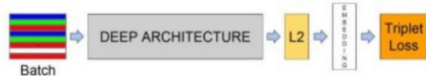
Fig. 2.Scroff et al.’s [3] FaceNet Model structure. The network consists of a batch input layer and a deep CNN followed by L2 normalization, which results in the face embedding. This is followed by the triplet loss during training.
