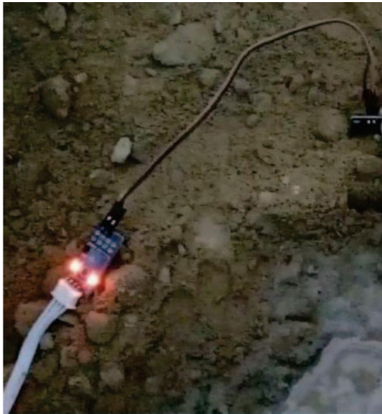
Fig.4. Soil moisture experiment for the second leakage scenario
