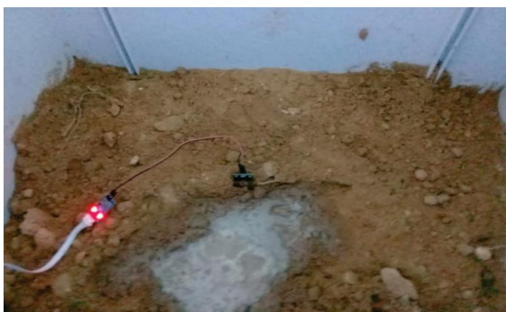
Fig.2. Soil moisture experiment for the first leakage scenario.
